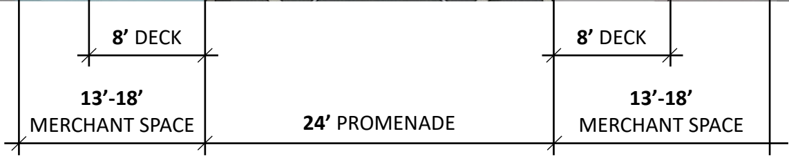
TYPICAL STREET SECTION – MERCHANT SPACE
