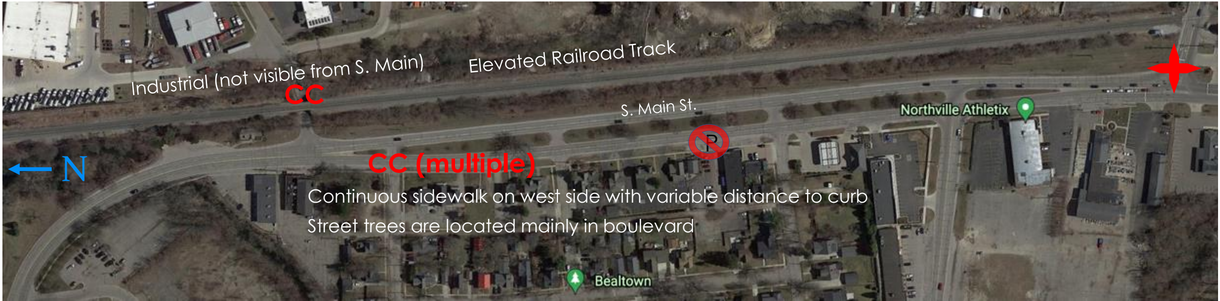
Figure 6B. Traffic volumes do not warrant 4 lane roads. Minimal infrastructure to protect pedestrians from vehicles. Wide lanes encourage speeds in excess of posted limits.
