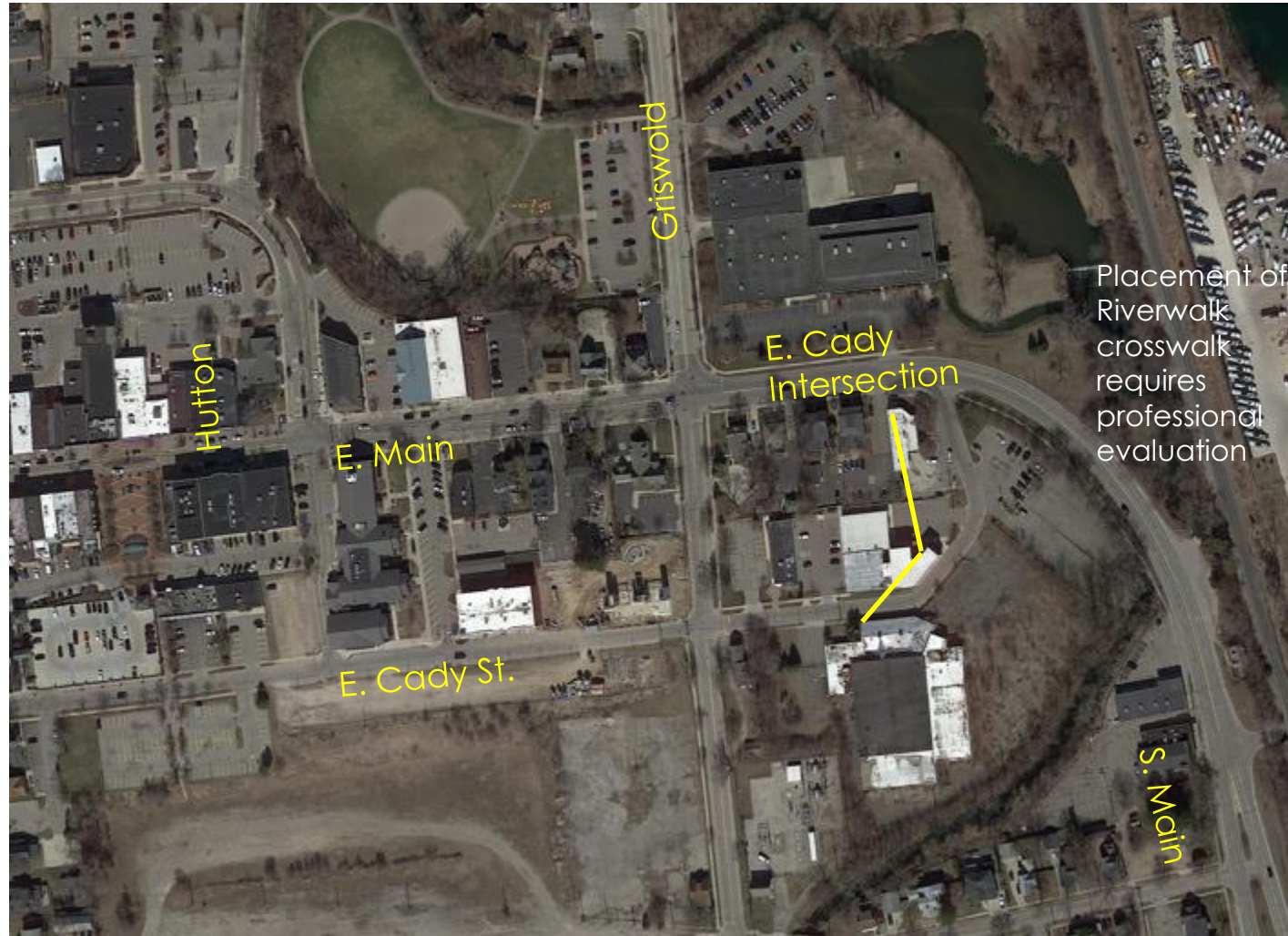
Figure 6C. The wide width of S. Main, coupled with a large curve radius, encourages higher-than-posted speeds. Limited visibility to E. Cady St. intersection creates less reaction time, which negatively affects pedestrian safety.
